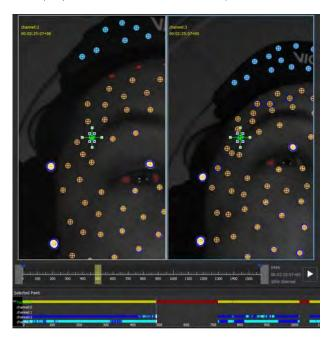
In this case, the marker point is attached to detections in channels 2 and 3 in the frame before the gap, so keyframe detections are added in channels 2 and 3 only.
