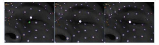
By the third example frame shown, the eye corner detection is almost completely occluded.
