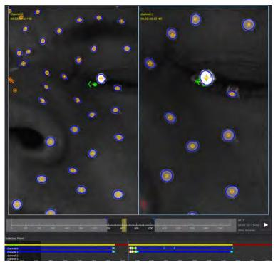
8. When you hit a failure case, navigate forward one frame, and add an additional keyframe at the last good tracking result by clicking Add Keyframe to Current Frame.
