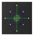
The blue box contains the pattern that you are tracking (the marker). Ensure it comfortably contains the marker. The green cross represents the comparison region, which is the area in adjacent frames that will be searched to find the pattern that is being matched (ie the marker). The green circle represents the middle of the pattern.
