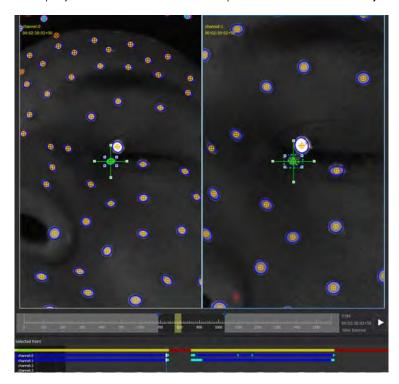
In this case, the marker point is attached to detections in channels 0 and 1 in the frame before the gap, so keyframe detections are added in channels 0 and 1 only.
